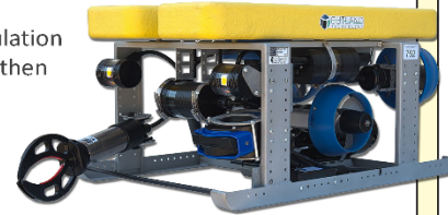
The Outland Technology ROV-2500, which is being used to record video footage for relative abundance indices.
